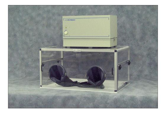
The front panel can be easily removed for access to the inside for cleaning. Floor is 1/2" thick, easy to clean, polyethylene. The HEPA filter captures particulate down to 0.3 microns in size, small enough to capture many bacteria, including Anthrax, which is 1 to 4 microns in size. An optional carbon filter may be added for additional protection. Unit is supplied with one pair of 14" 15 mil neoprene gloves and one pair of 15 mil neoprene glovebox gloves (please state sizes required S, M, L).
